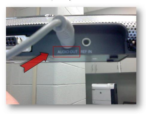
Connect to computer ports – USB and Audio cable are connected.
